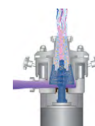
Module Colloid / Cone mill MK / MKO Wet-milling using a milling tool with an adjustable gap. Emulsification (MK) and de-agglomeration (MKO) of viscous products.
